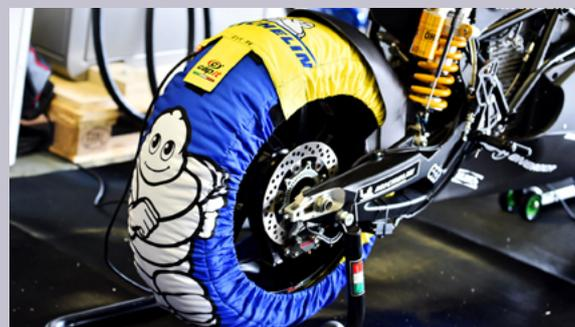
✓ Every machine is delivered with 2 sets of tyre warmers for use with slick tyres, and 1 set of tyres warmers for use with rain tyres.
